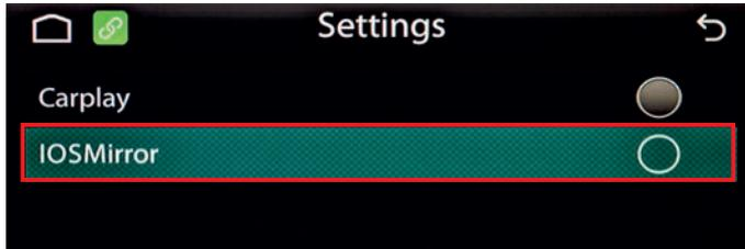
3. After selecting IOSMirror, connect the Apple data cable (original cable) to the USB cable installed in the main unit, it will appear on the phone as shown in the picture. Click "Trust", and Airplay will work successfully.
